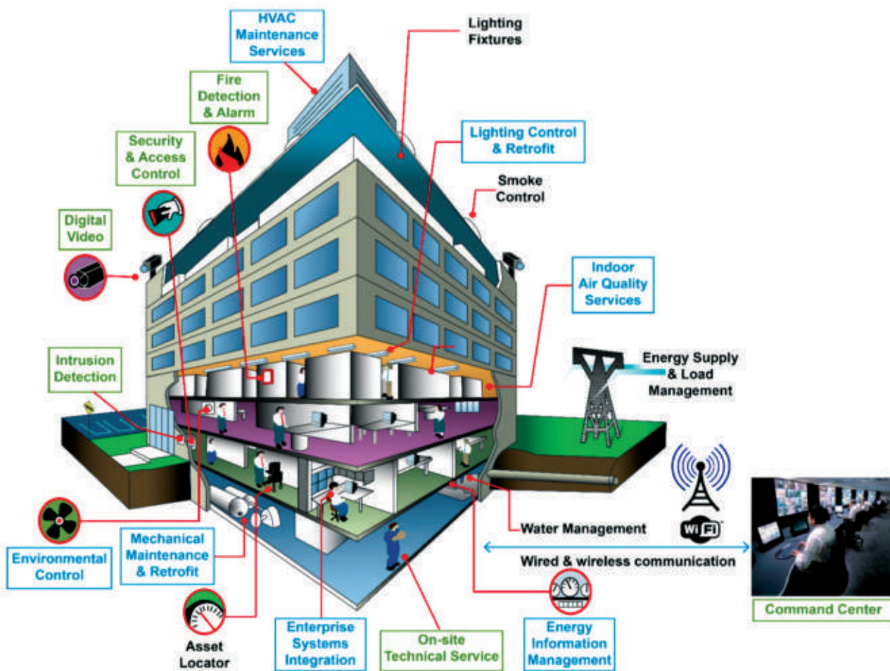
Building Automation System (BAS)
