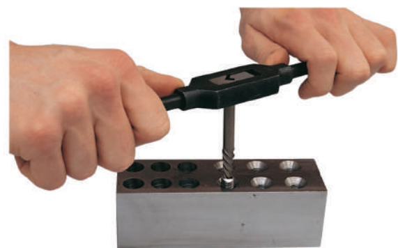
Figure 14 Type of Tap and working on Tap
